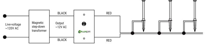
Note: All 12V LED devices will dim differently. The trim pot switch will need to be adjusted for wattage loads and or 12V dimmable LED products. This LED dimmer is made for 12VAC Transformers only. Do not exceed 96 WATTS on the field load.
